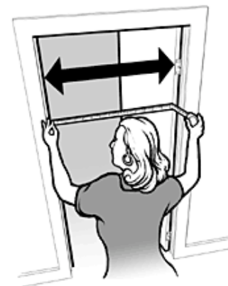
Open the door 90 degrees. Measure between the edge of the doorway on one side, and the inside edge of the door frame on the other side. This must be at least 32 inches wide.
